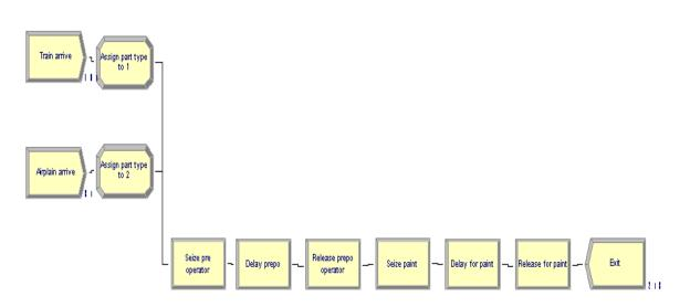
Figure 2 Scenario models in Arena Simulation
